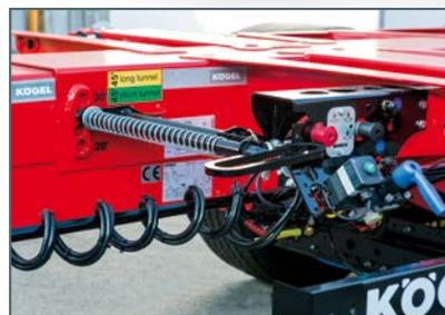
For a **longer lifespan,** the **centre extension (extendible to four different positions)** features a **low-maintenance guide** on special plastic sliders and two extension rollers. The rear extension **is designed along the same lines.** This can **be quickly set** to one of seven possible positions using a hand crank
