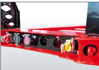
**The air and light console is housed in a protective recess in the front extension,** significantly increasing the free space around the tractor unit connection cables
