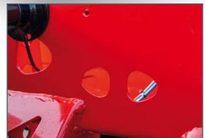
**Permanent protection from corrosion** thanks to the nano-ceramic technology plus cathodic dip-paint coating followed by UV coating of the entire vehicle frame
