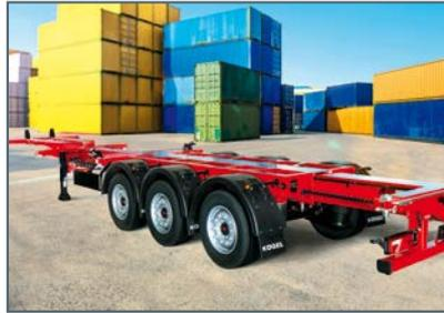
**One of the lightest container chassis on the market offers maximum economic efficiency.** With a low tare weight starting at 4,250kg (with individual equipment), an approx. payload of more than 36,520kg is possible
