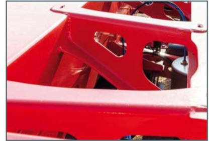
**Optimum stress distribution** thanks to the elliptical lightweight perforations
