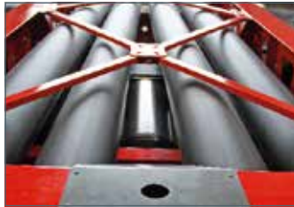
Stowage for hose pipes
