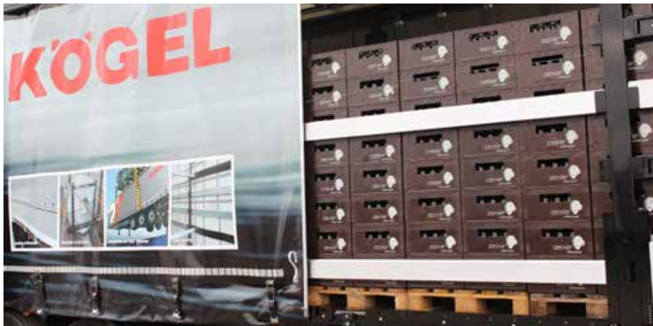
Single-level beverage transport with two rows of lattices Twin-level beverage transport with three rows of lattices
